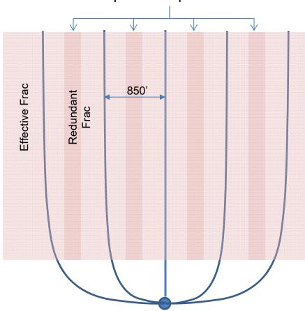
Drilling at 850' spacing When optimal is 1050'
