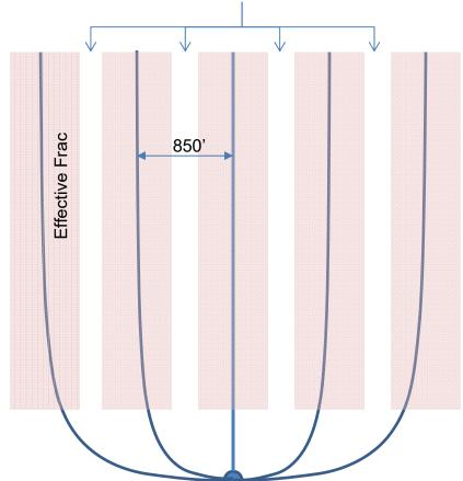
Drilling at 850' spacing When optimal is 650'
